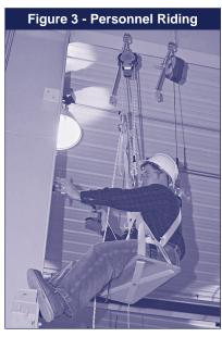
a full body harness or rescue sling, anchorage connector (i.e. carabiner, etc.) and the Rollgliss R350. See Figure 4.
